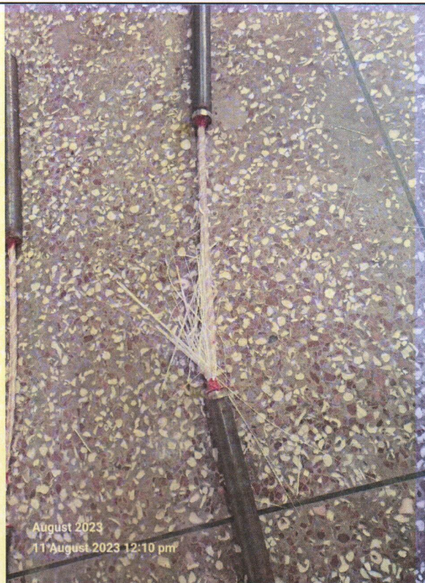
Description: FRACTURED SAMPLE; AFTER TEST
