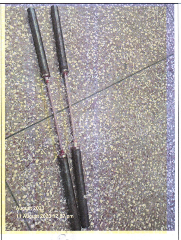
Description: 7MM REBAR SAMPLES; AFTER TEST
