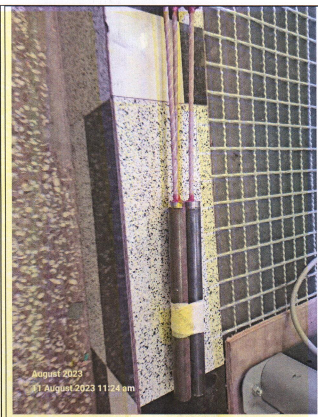
Description: 7MM REBAR SAMPLES; BEFORE TEST
